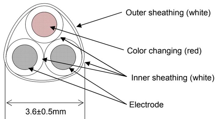
Fig. 2: Cross-section Diagram of the AD-HS Sensor
