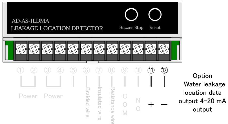
Drawing 7 Water Leakage Location Data Output Connection
