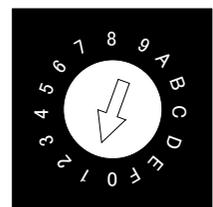
To set a Modbus Address, operate the rotary switch of the detector.
