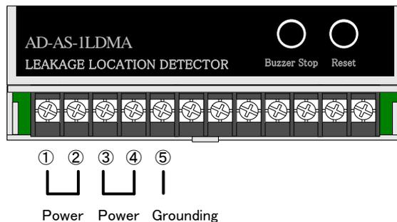
Drawing 3 Layout Drawing of Terminal Block
