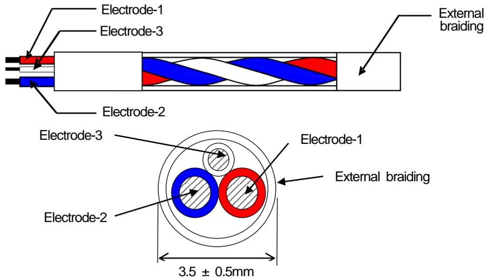
Drawing 4 AD-LS Sensor Structure
