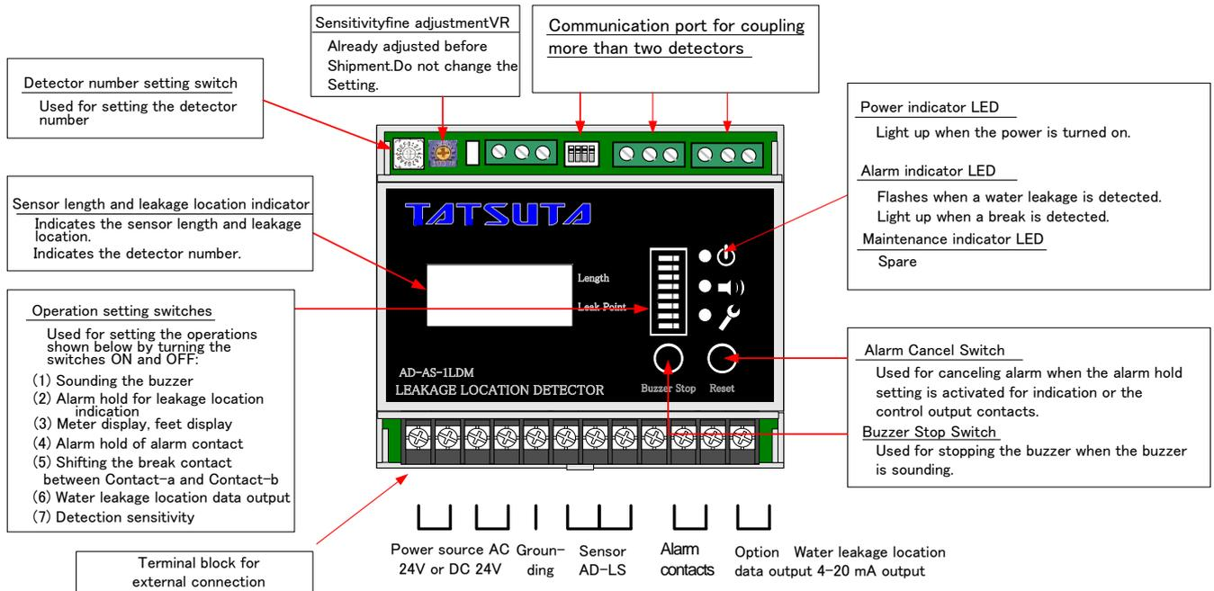
Drawing 1 Explanation of Individual Parts of Water Leakage Location Detector
