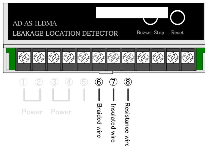
Drawing 5 Terminal Block for Sensor Connection
