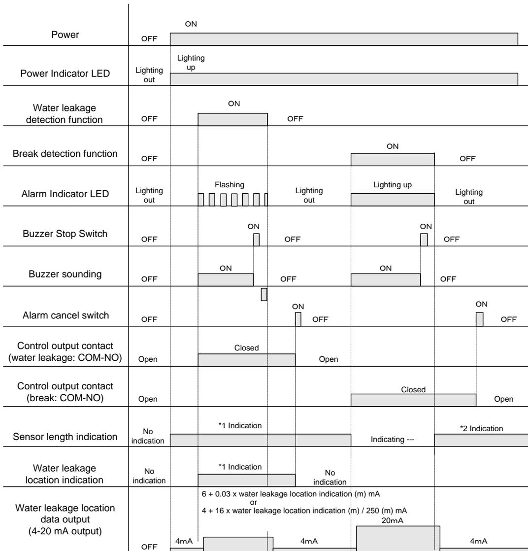
\*1 The sensor length and the water leakage location are indicated alternately. (Refer to Attached Drawing 4)
