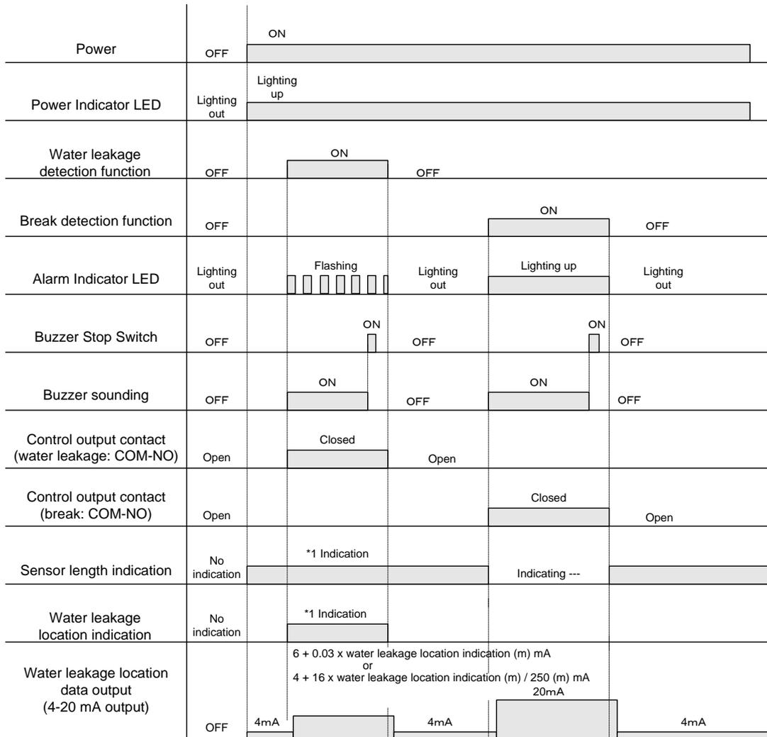
\*1 The sensor length and the water leakage location is indicated alternately.
