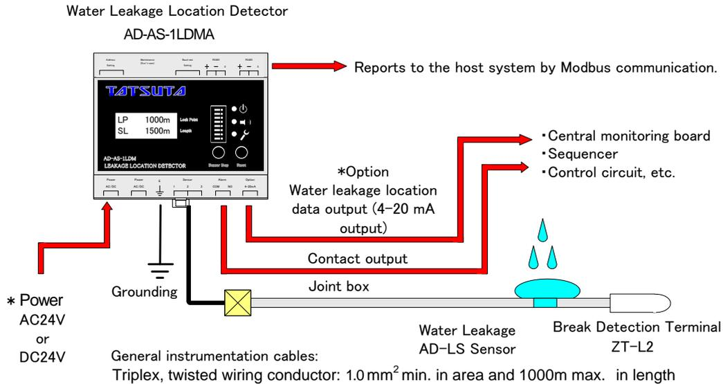
Drawing 2 Water Leakage Location Detecting System
