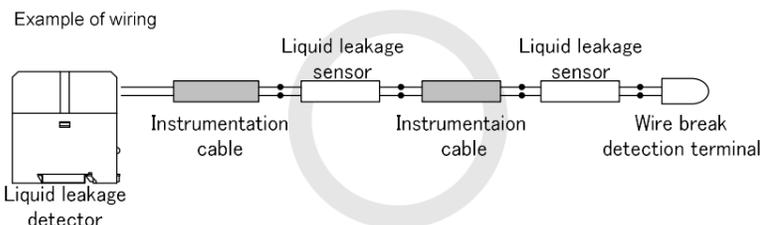
To extend the sensor, connect the instrumentation cable in series.
