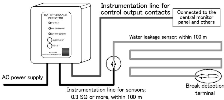
Fig.2 Typical detecting system configuration
