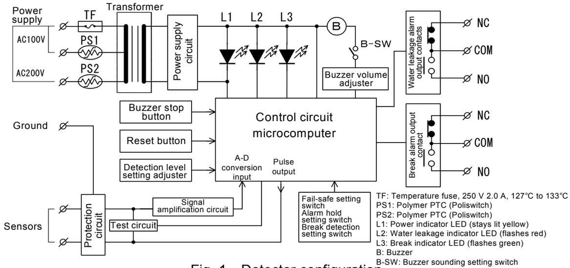
Fig. 1 Detector configuration
