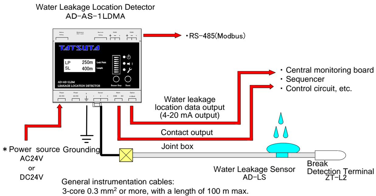
Drawing 1 Water Leakage Location Detecting System
