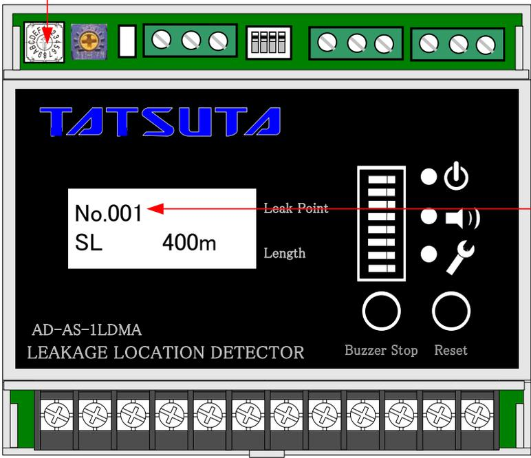
To set a Modbus Address, operate the rotary switch of the detector.
