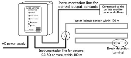
Fig.2 Typical detecting system configuration
